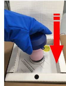
Replace shippo plug. Shippo plug can be used to help insert Tyvek bag down into storage well.
