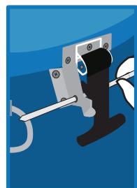
Thread end of zip-tie through the hole on the other side of the metal hardware.
