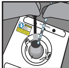
Safely place the cane with the secured goblets or vials and sleeve into the canister and lower into the dewar.
