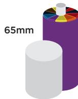
If the straw/commodity is loaded in a 65mm goblet (Daisy Goblet), place the Goblet onto the lifter and lower the commodity into the dewar.
