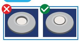
The center buttons will eject and appear flush when the latches are successfully engaged.
